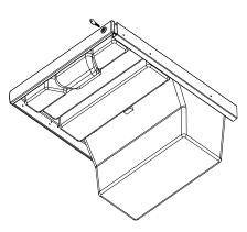
3. Locate the Rail Release Levers. Slide your hand along the inside of the rail along the drawer.
